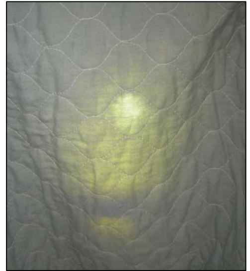
Light Evaluation Test showing a thin spot on the thermal liner
