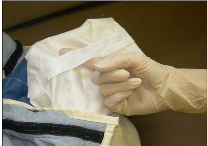
Loose moisture barrier seam tape
