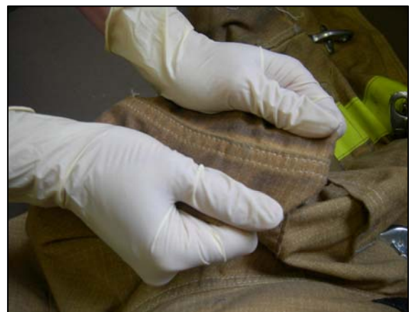
Discoloration on outer shell caused by thermal damage
