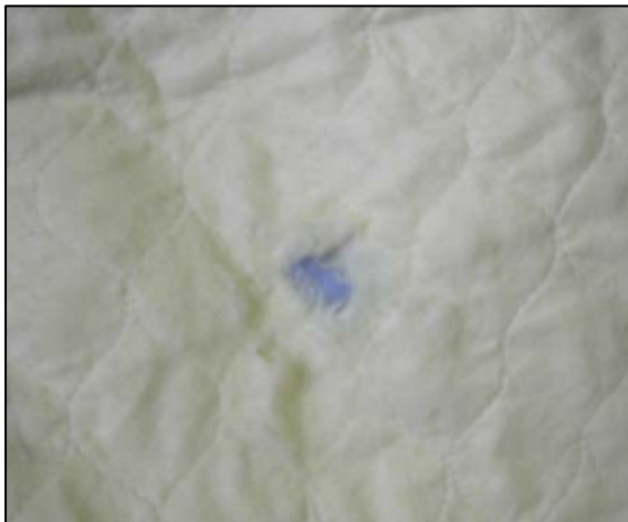
Shifting of thermal liner material (batting)
